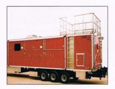
numbers of contaminated people. The units allow victims to enter on a trailer's dirty side and quickly exit on the clean side, free of contaminants. Showers and drain systems are designed to minimize cross-contamination, and water is contained for disposal. Air in the units is filtered.
