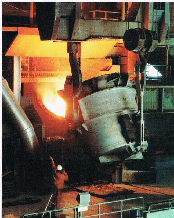
Hot metal pours from ladle into BOF at Edeltahl Witten-Krefeld GmbH.
